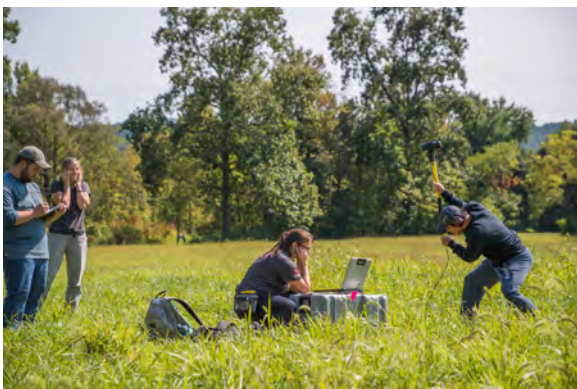
Anne Meltzer's undergraduate seismology class conducting a seismic reflection survey last fall in Zionsville, PA.
