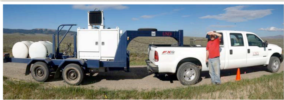
The seismic source IVI miniviv T-7000, used for energizing during the data acquisition.
